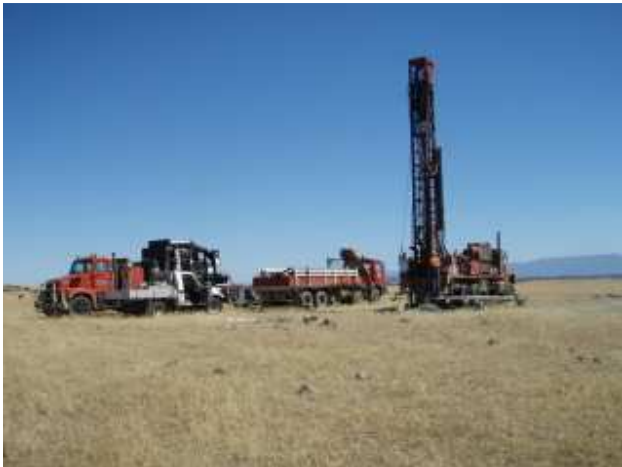
Plate 3. Pre-collar drilling at Epping.
